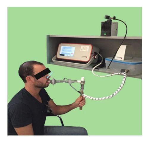
compact ( $92 \times 190 \times 255$  mm) and lightweight (2.3 kg) portable olfactory system, consisting of a gas sampling unit and a sensor array. Using a pattern recognition software (Win Muster v. 1.6.2), the PEN3 allows visualization and analysis of the data and works using filtered ambient air during the cleaning step or dilute gas during sampling with a maximum flow rate of 600 ml/min.
